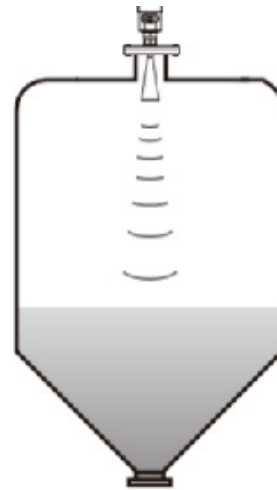
Figure 16: The conical tank with flat top can be installed in the middle of the tank top to ensure that the measurement to the conical bottom.
